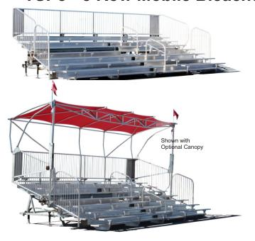
Reduced towing weight and increased maneuverability make these eight-row bleachers ideal for use on sports fields and other soft-surface applications. Multiple frame-mounted leveling-support jacks distribute seating loads over a wide area. Aluminum seat and footboards offer a high degree of weather resistance, promoting year-round use. A retractable towing tongue reduces the overall length when set up, while eliminating a tripping hazard.
